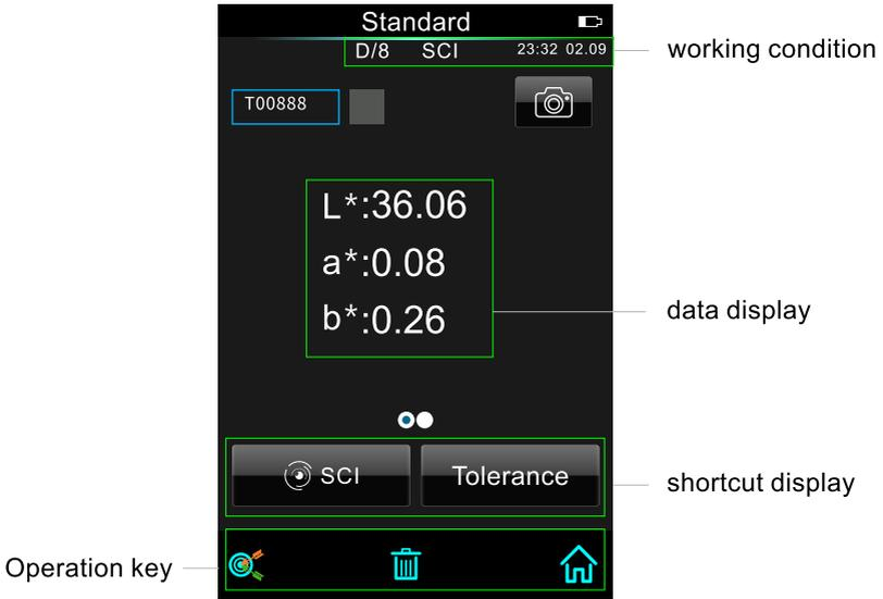
Figure 6 Standard Measurement Interface
