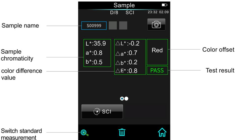
Figure 14 sample measurement interface
