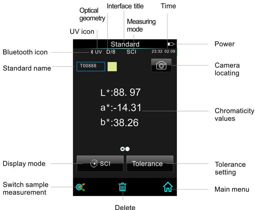
Figure 11 Standard Measurement
